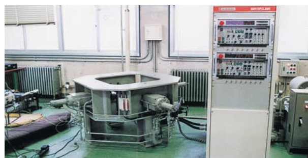
大型二軸加振機 Large double-shafted agitator/mixer 平面二軸の動的負荷試験を行う Performing dynamic load
